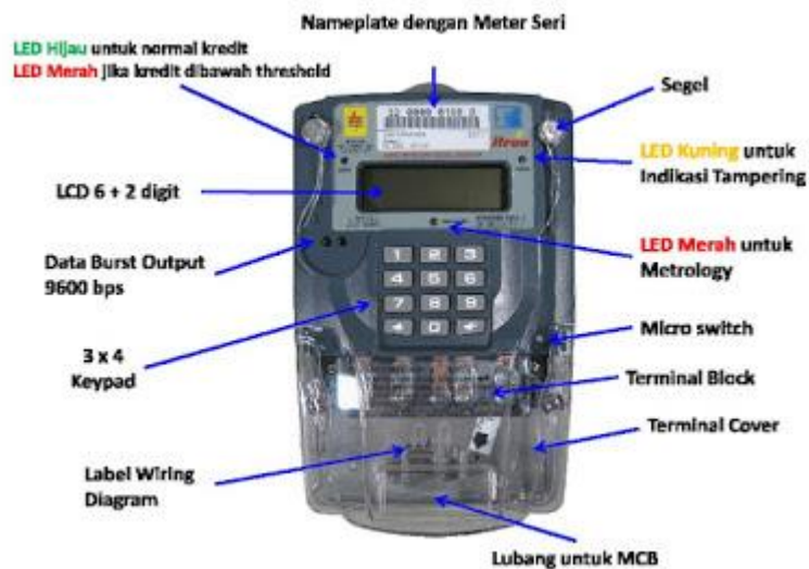
Gambar 5.7 Bagian-bagian KWH meter Digital
