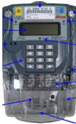
Gambar 5.5 KWH Meter Digital
