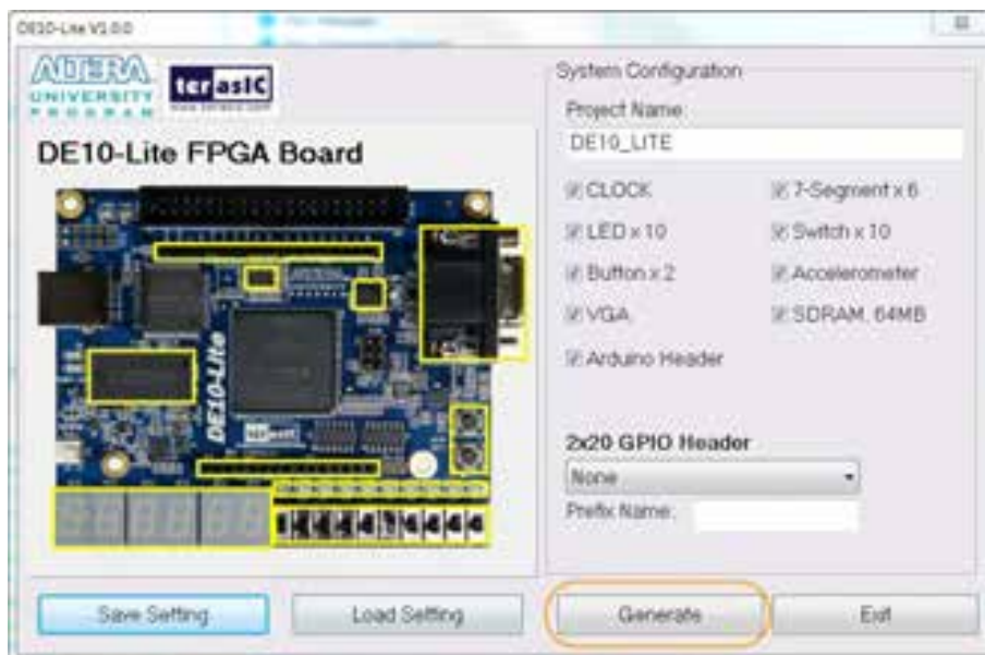
Figure 4-7 Generate Quartus Project
