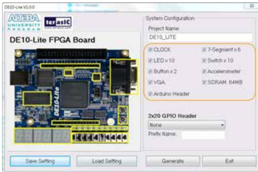
Figure 4-4 System configuration group
