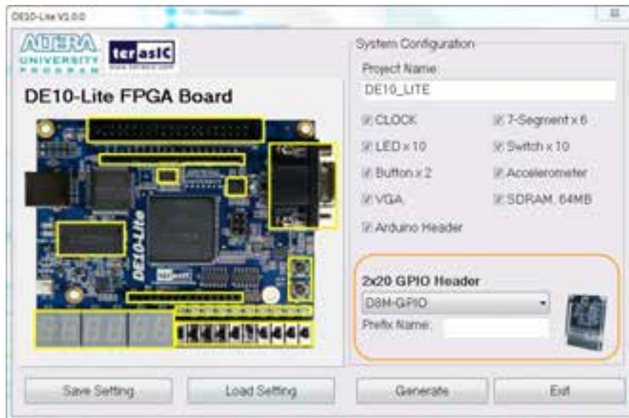
Figure 4-5 GPIO expansion group
