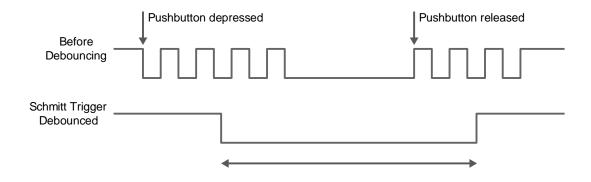
Figure 3-4 Pushbuttons debouncing
