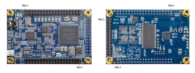
Figure 3-12 Pin1 locations of the 2x13 header
