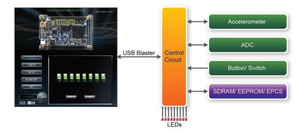
Figure 4-2 The DE0-Nano Control Panel concept
