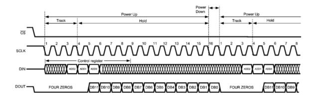
Figure 8-11 4-wire SPI Timing Diagram
