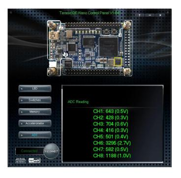
Figure 4-7 ADC Readings
