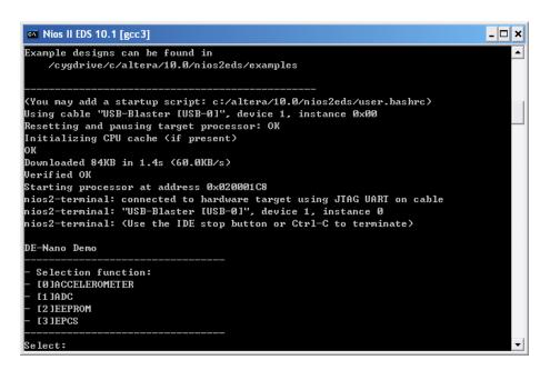
• Input "0" to start the accelerometer demo. The demo starts by displaying the accelerometer's chip ID, and then continues by displaying the X/Y/Z values every 1.0 second. To terminate the demo, press KEY0 or KEY1 on the DE0-Nano board. Upon exiting the demo, the selection menu will be displayed.
