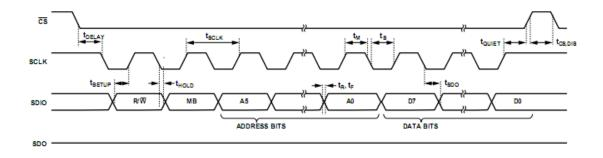
Figure 8-10 3-wire SPI Timing Diagram
