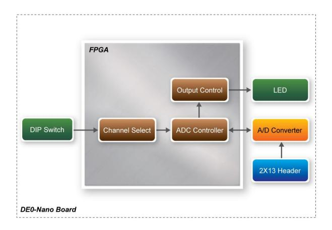
Figure 8-3 ADC Reading Block Diagram
