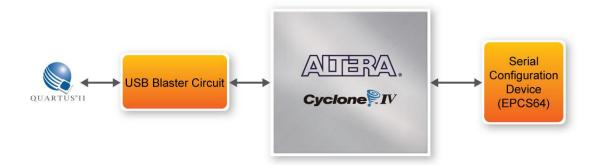
Figure 3-1 Programming a serial configuration device with serial flash loader solution
