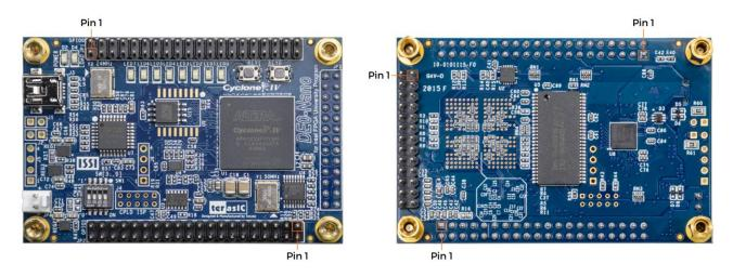
Figure 3-9 Pin1 locations of the GPIO expansion headers
