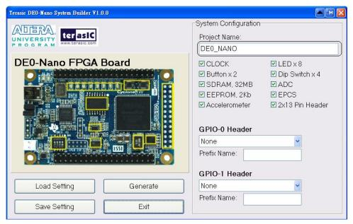
Figure 5-3 The DE0-Nano Board Type and Project Name
