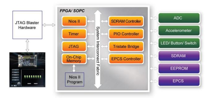
Figure 4-8 The block diagram of the DE0-Nano Control Panel
