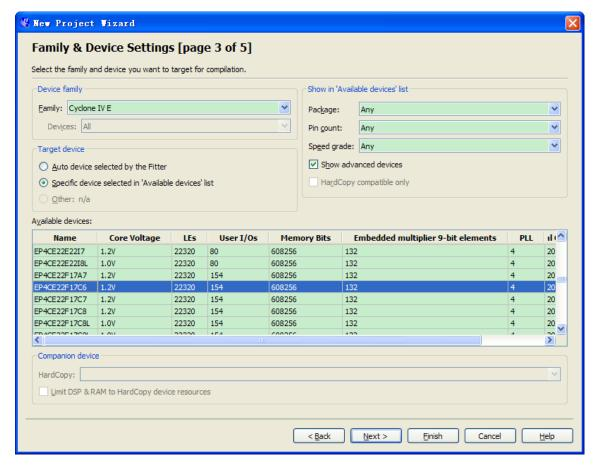
Figure 6-10 Specify the Device Example
