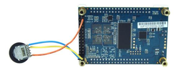
Figure 8-5 ADC Reading hardware setup
