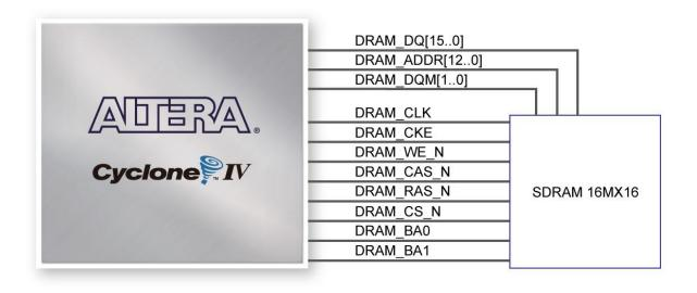
Figure 3-6 Connections between FPGA and SDRAM
