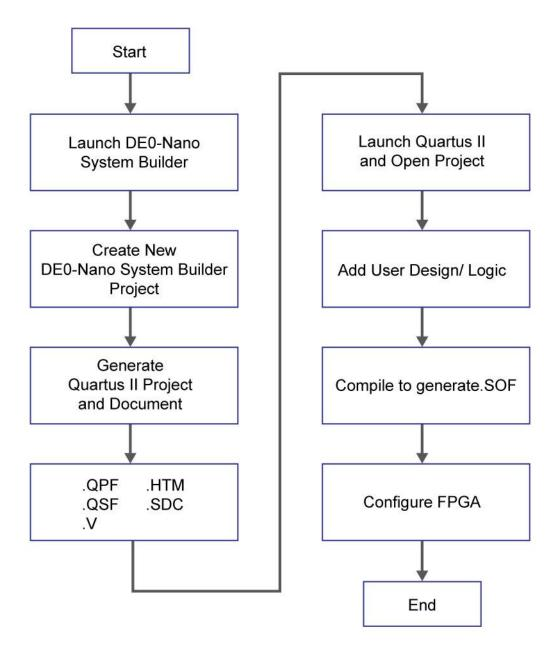
Figure 5-1 The general design flow of building a design
