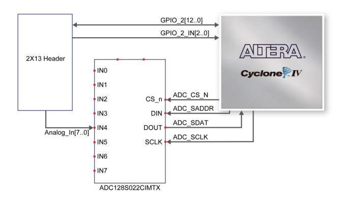
Figure 3-11 Wiring for 2x13 header and A/D converter
