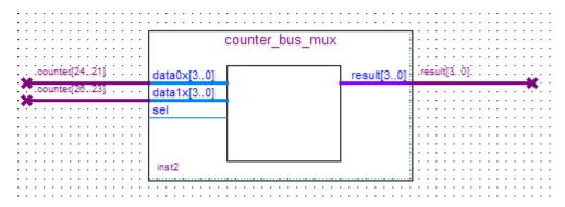
Figure 6-37 Renamed counter\_bus\_mux Bus Lines
