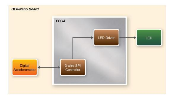
Figure 8-14 G-Sensor block diagram
