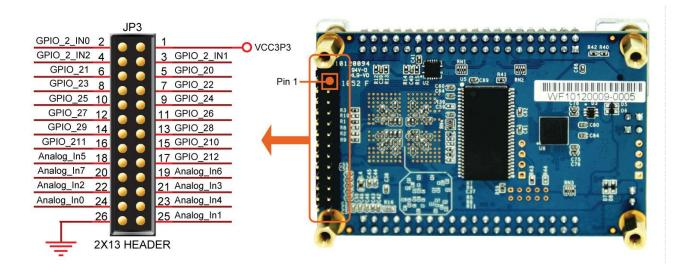
Figure 3-10 Pin distribution of the 2x13 Header
