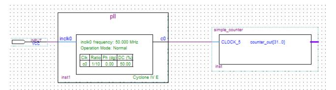
Figure 6-29 Connecting the PLL symbol and Input port
