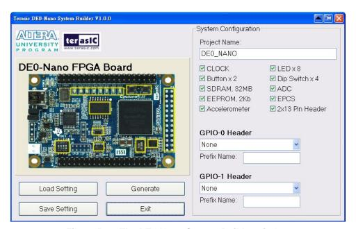
Figure 5-2 The DE0-Nano System Builder window
