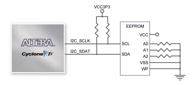
Figure 3-7 Connections between FPGA and EEPROM
