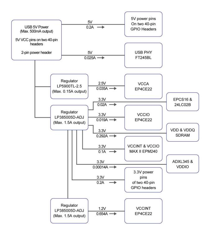
Figure 3-16 DE0-Nano Power Distribution System
