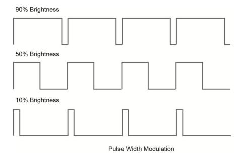
Figure 8-2 Pulse Width Modulation
