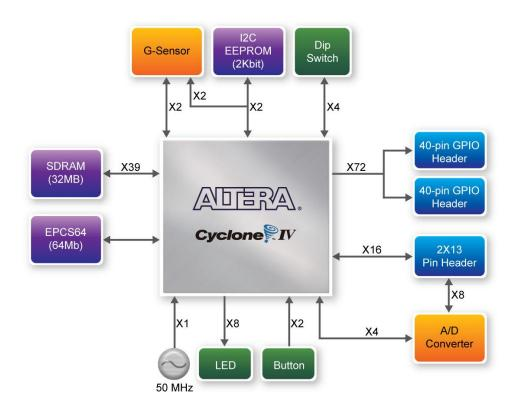
Figure 2-3 Block diagram of DE0-Nano Board
