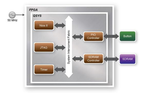
Figure 8-15 Block diagram of the SDRAM Basic Demonstration
