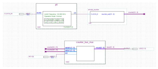
Figure 6-40 Adding the KEY [0] Input Pin
