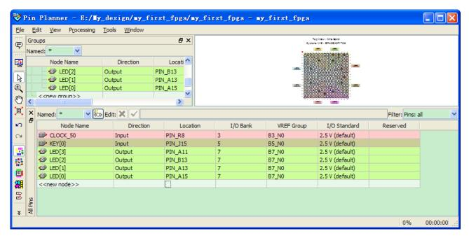
Figure 6-42 Completed Pin Planning Example
