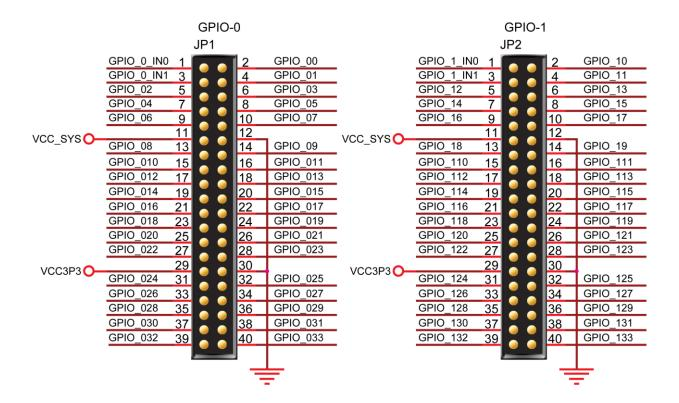
Figure 3-8 Pin arrangement of the GPIO expansion headers
