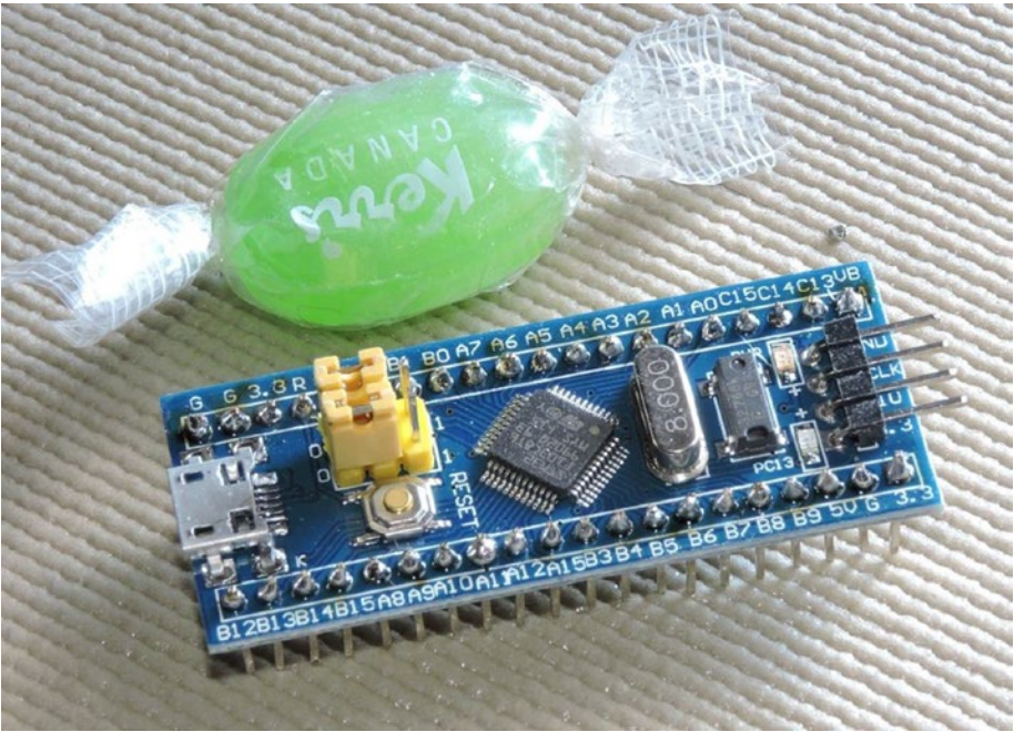
Figure 1-1. The STM32F103C8T6 PCB (printed circuit board) with the header strips soldered in, often referred to as the “blue pill”
