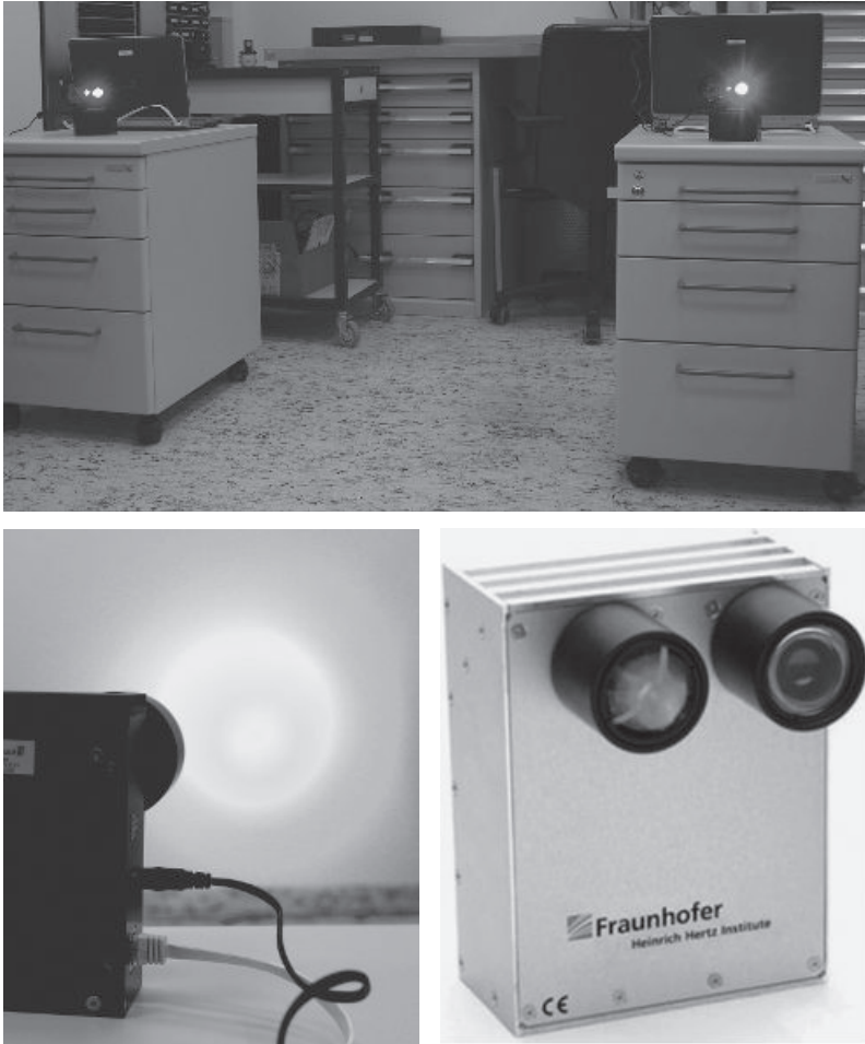
Figure 8.16 (Top): Two bidirectional transceivers communicating via a diffuse link. Different colors are used for down and uplink as an example, but also the same colors can be used. (Bottom left): View of the diffusing spot of the link at a (standard painted) wall at a distance of up to \sim 3 m from the transceivers. The overall link length is about 6 m. (Bottom right): New generation of bidirectional transceiver with a form factor of 87 \times 114 \times 42 mm 3 (without lenses).
