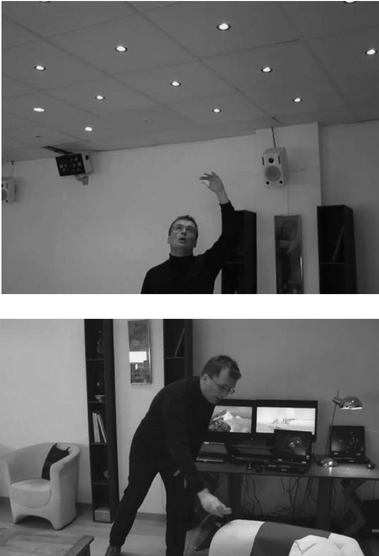
Figure 8.15 The first public demonstration of a high-speed VLC system using DMT modulation for broadcasting multiple video streams at a data rate of 100 Mbit/s (125 Mbit/s gross data rate at PHY layer). ( Top ) Array of VLC transmitters on the ceiling; ( bottom ) mobile receiver device consisting of a photodetector and an amplifier for forwarding the signal to the demodulator and further to the video screens.
