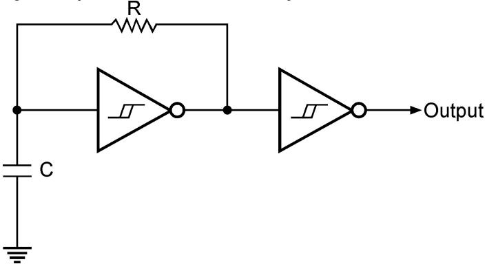
Figure 4.54 Schmitt inverter based oscillator.
