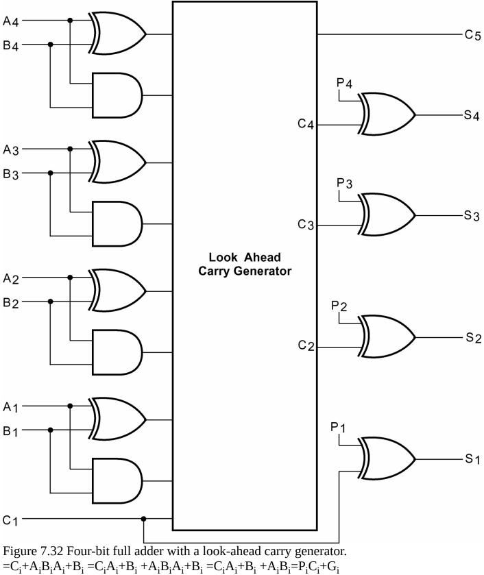
$$\begin{split} =& C_i + A_i B_i A_i + B_i = C_i A_i + B_i + A_i B_i A_i + B_i = C_i A_i + B_i + A_i B_i = P_i C_i + C_i \\ S_i =& A_i \oplus B_i \oplus C_i = A_i B_i + A_i B_i \oplus C_i \\ Also \\ P_i G_i \oplus C_i =& A_i + B_i A_i B_i \oplus C_i \\ =& A_i + B_i A_i + B_i \oplus C_i = A_i B_i + A_i B_i \oplus C_i \\ Therefore, S_i =& P_i G_i \oplus C_i. \end{split}$$
