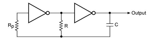
(b) Figure 4.53 Square-wave oscillator with external components.
