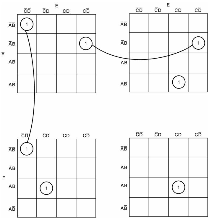
Figure 6.16 Multiple Karnaugh map for a six-variable Boolean function. Solution
