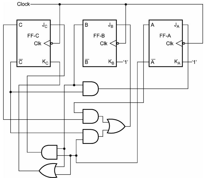
Figure 11.31 Hardware implementation of the counter circuit (example 11.9). Table 11.13 Example 11.9. Present state Next state Inputs C B A C BAJ<sub>A</sub> K<sub>A</sub> J<sub>B</sub> K<sub>B</sub> J<sub>C</sub> K<sub>C</sub>
