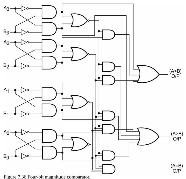
(7.27) respectively representA>B andA<B conditions. Figure 7.36 shows the logic diagram of a four-bit magnitude comparator.
