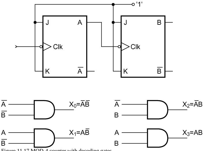
Figure 11.17 MOD-4 counter with decoding gates.
