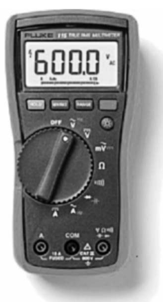
Figure 16.9 Handheld digital multimeter. Reproduced with permission of Fluke Corporation.
