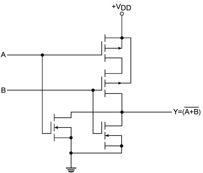
Figure 5.52 Unbuffered two-input NOR.
