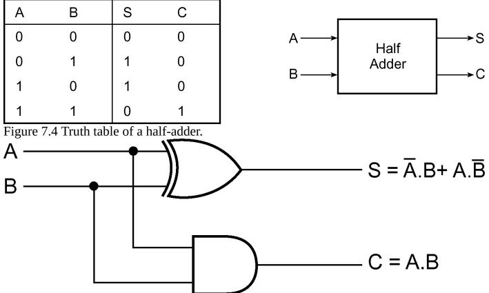
Figure 7.5 Logic implementation of a half-adder.
