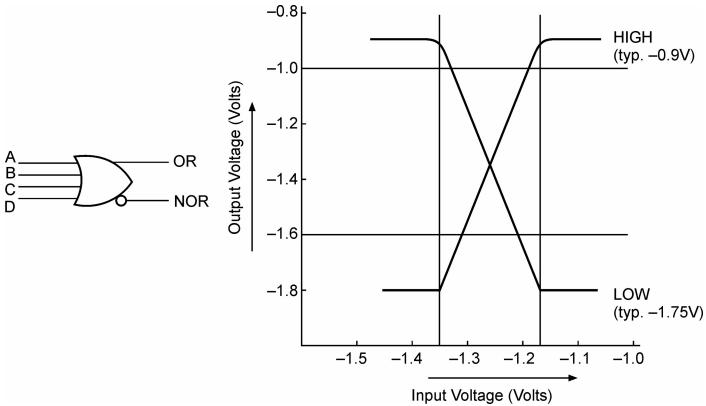
Figure 5.33 ECL input/output characteristics.
