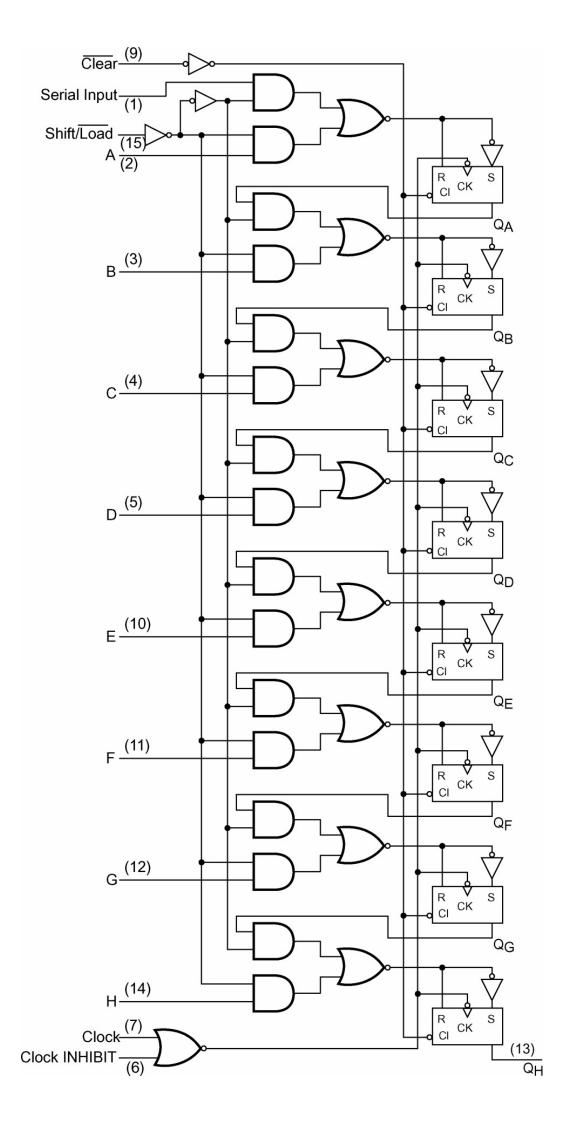
Figure 11.40 Logic diagram of 74166.
