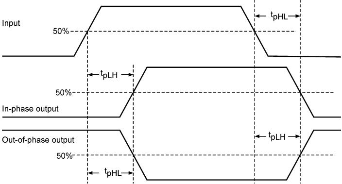
Figure 5.4 Propagation delay parameters.
