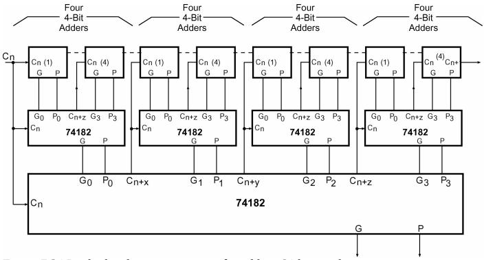
Figure 7.34 Look-ahead carry generation for adding 64-bit numbers. 7.7 Arithmetic Logic Unit (ALU)
