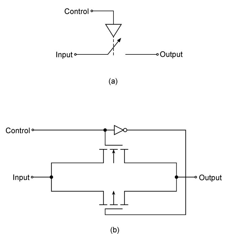
Figure 5.45 Transmission gate.
