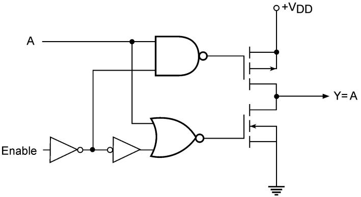
Figure 5.48 Tristate buffer in CMOS.
