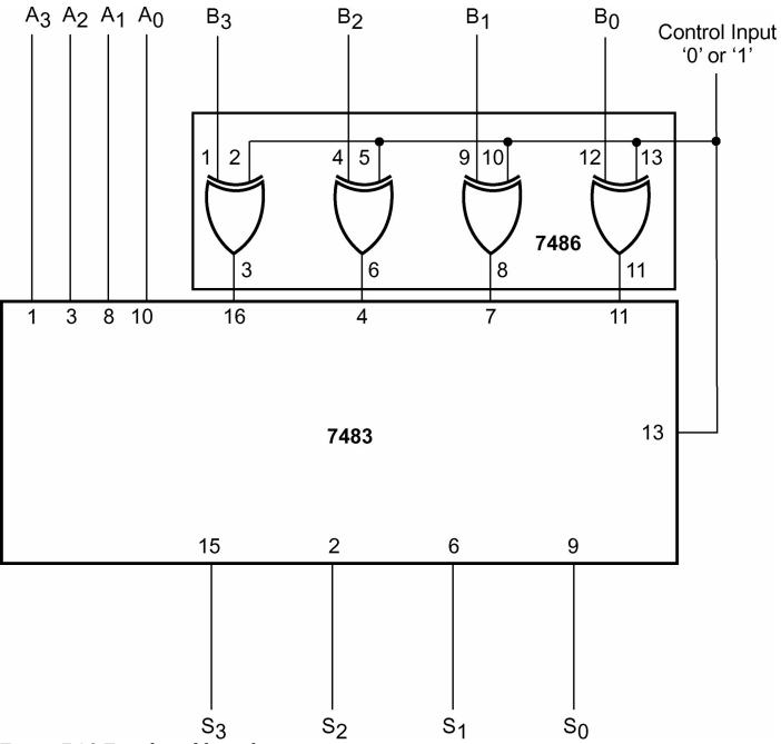
Figure 7.20 Four-bit adder-subtractor.
