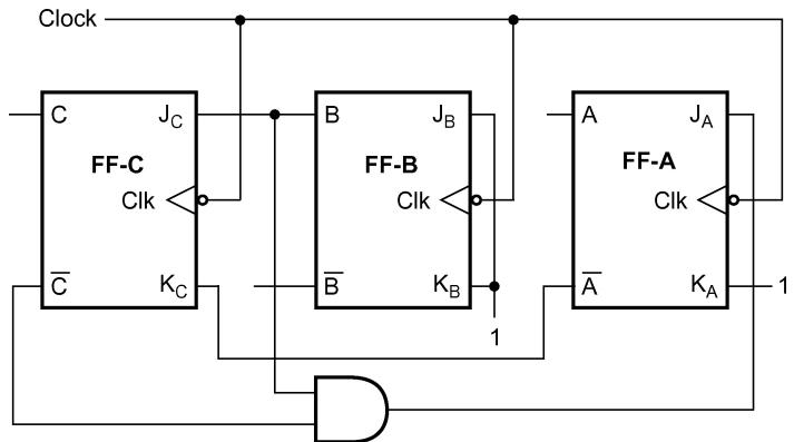
Figure 11.33 Hardware implementation of the counter circuit (example 11.9).
