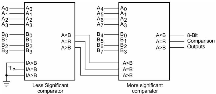
Figure 7.37 Cascading of individual magnitude comparators. Table 7.2 Functional table of IC 7485 or IC 4585.
