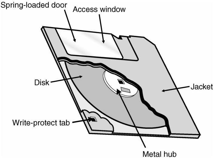
Figure 15.34 Important parts of a floppy disk.
