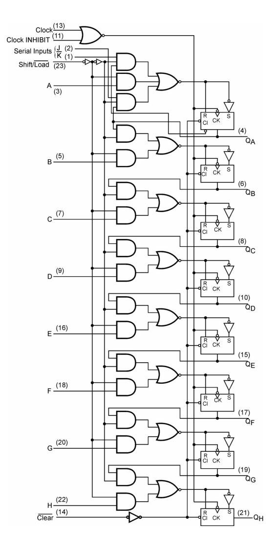
Figure 11.42 Logic diagram of IC 74199.
