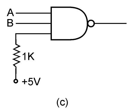
Figure 5.24 Handling unused inputs of AND and NAND gates.
