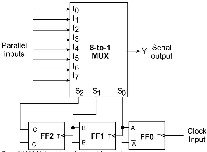
Figure 8.11 Multiplexer for parallel-to-serial conversion. 8.1.3 Multiplexers for Parallel-to-Serial Data Conversion
