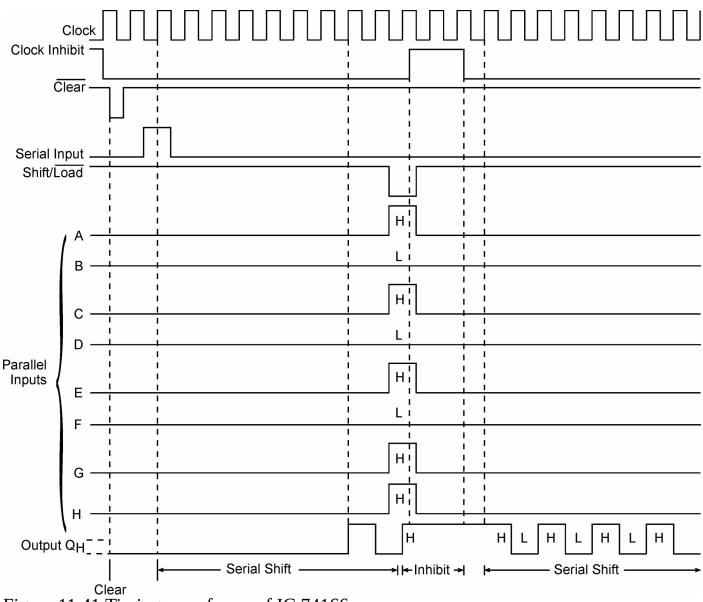
Figure 11.41 Timing waveforms of IC 74166. 11.12.5 Bidirectional Shift Register
