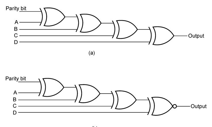
(b) Figure 4.51 Parity check using EX-OR and EX-NOR gates. 4.13.4 Inverter
