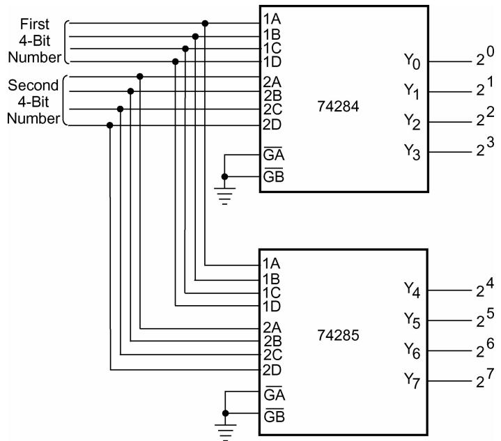
Figure 7.35  $4 \times 4$  bit multiplier.
