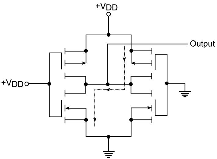
Figure 5.46 CMOS inverters with shorted outputs.
