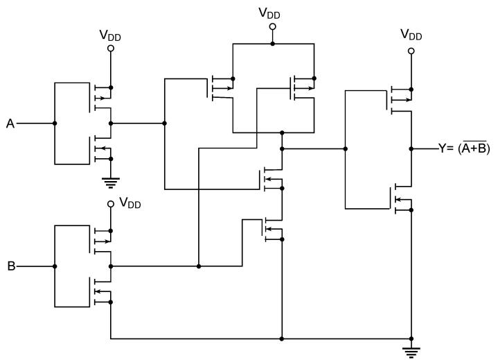
Figure 5.51 Buffered two-input NOR.
