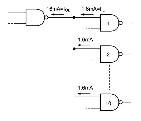
Figure 5.2 Input and output current specifications.
