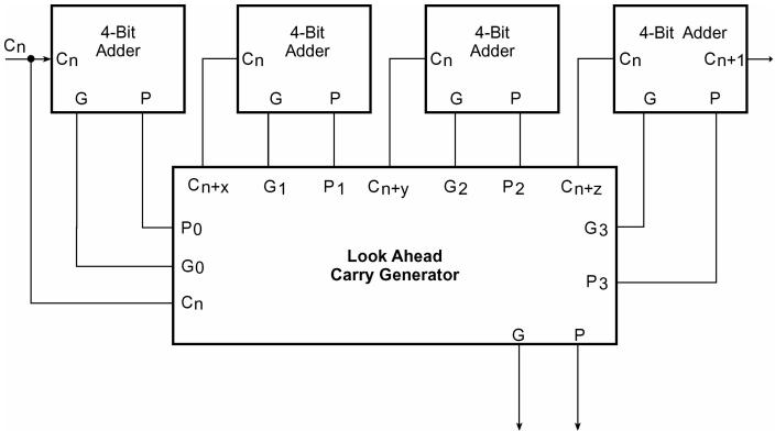
Figure 7.33 IC 74182 interfaced with four four-bit adders.
