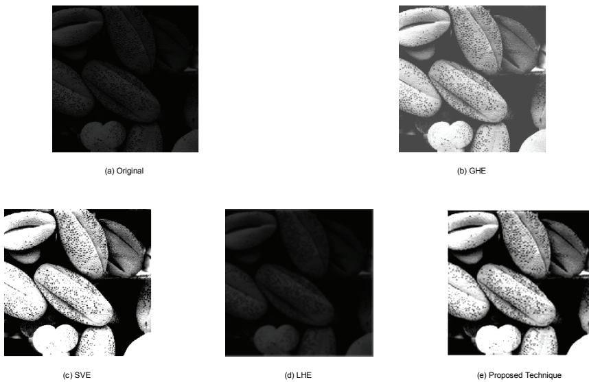
Fig. 3. (a) Low contrast image, Equalized image using: (b) GHE, (c) SVE, (d) LHE, and (e) the proposed technique.
