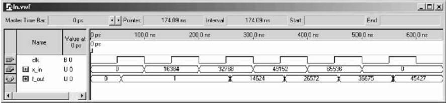
Fig. 2.54. VHDL simulation of the \ln(1+x) function approximation for the values x = 0, x = 0.25 = 16384/65536, x = 0.5 = 32768/65536, x = 0.75 = 49152/65536, x = 1.0 = 65536/65536 .
